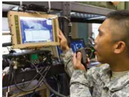
Figure 1 Bus-less embedded computer form factors like Pico-ITX, Min-ITX and Thin-Mini-ITX are particularly attractive in space-constrained military applications that require advanced graphics for user interfaces.
