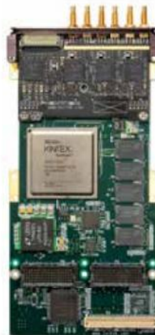
Jade Model 71861 XMC module, also available in VPX, PCIe, cPCI and AMC with rugged options.
